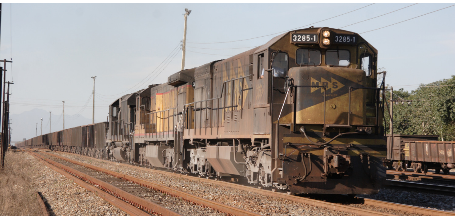
▼ MRS Logística SA No. 3285, a General Electric U23c design unit, leads GE C36M type No. 3879, formerly in use with Union Pacific, and Macosa SD40-2 No. 5243 on 4th August 2007. The trio are departing from Brisamar yard with an iron ore train for export from the Guaíba Island terminal.
