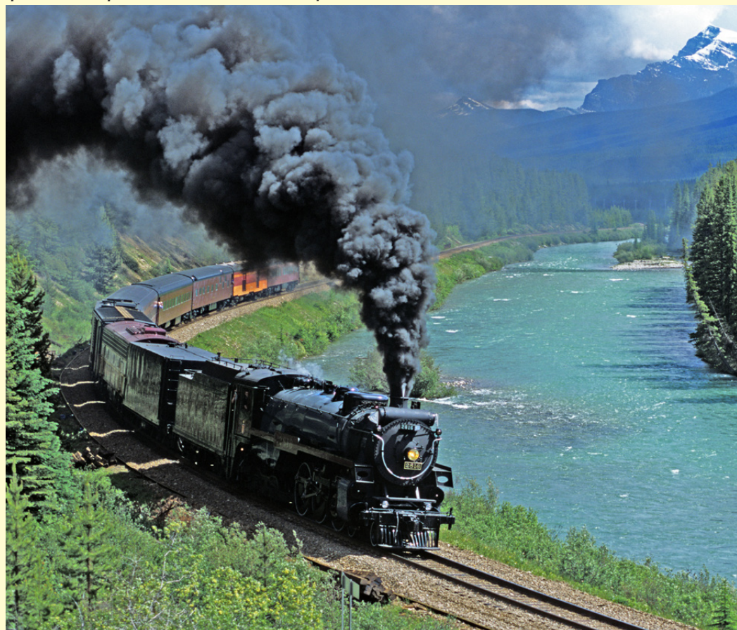
▼ Canadian Pacific operate Royal Hudson No. 2816 Empress , a 1930s-built 4-6-4 that is oil-fired to cut down the fire risk in the various National Parks that the line runs through. On 29th June 2005, the loco is performing a rather spectacular run-past at the well-known location of Morants Curve.
