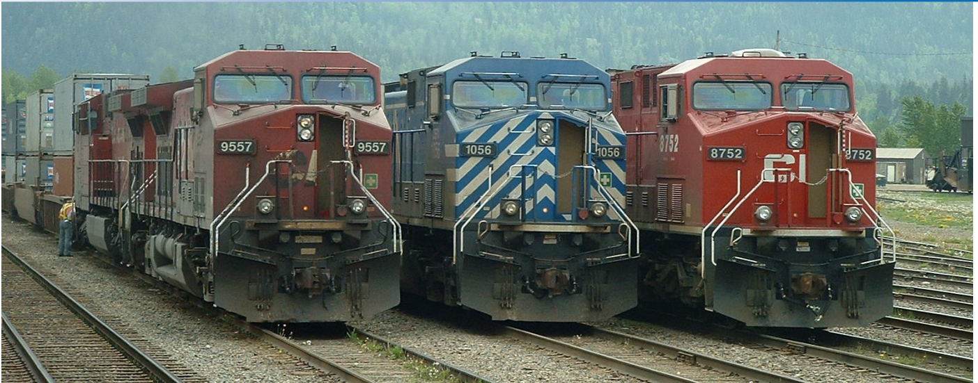
▲ The scene at Revelstoke Yard, British Columbia, Canada, on 16th December 2007, as three freights line up to head westwards to Kamloops and over the 'Kicking Horse' pass. From left to right are Canadian Pacific General Electric AC4400CW No. 9557, lease power from CEFX in the form of General Electric-built AC4400CW power No. 1056 and Canadian Pacific General Electric ES44AC No. 8752. Ray Barber
