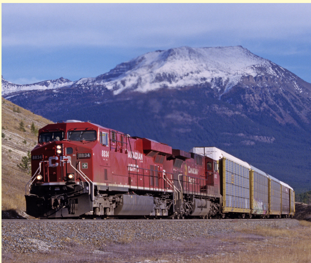
◀ An ES44AC No. 8834 leads AC4400CW No. 9612 on the climb from Lake Louise to Divide with a westbound Intermodal bound for Vancouver on 14th October 2007. The wagons behind the locos are called Autoracks, which carry cars on three levels.
