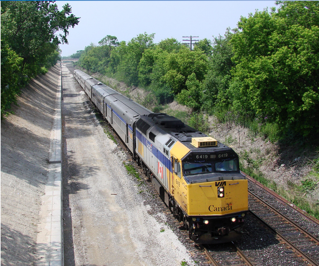
▲ One of VIA Rail's EMD F-40PH design locomotives, No. 6419 powers through Scarborough, Ontario, Canada. This is one of the locomotives that will be rebuilt under the terms of the contract. Richard Usecwicz
