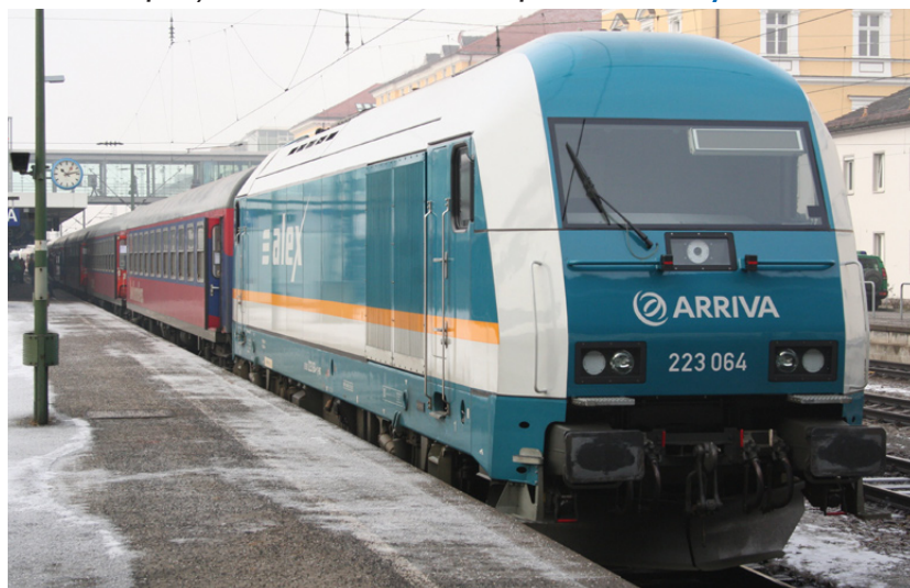
▼ GERMANY: Arriva Class 223 No. 223064 waits to depart Regensburg Hbf on 11th January, with the 08.44 München Hbf - Praha HI N service. Operator Alex took over the operation of these services from December 2007 using hired in coaches, and Class 183 electrics between München and Regensburg. Class 223 diesels work from Regensburg via Schwandorf (where a reversal takes place) to Furth i Wald on the Czech Republic border. Andy Pratt
