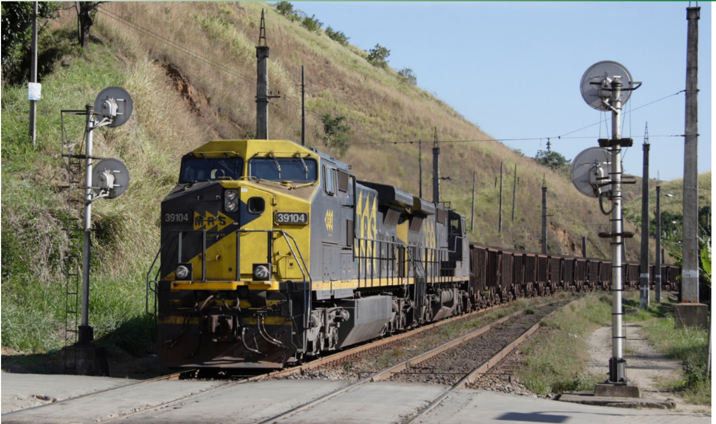
▲ On the 1.6-metre broad-gauge network MRS Logística SA-operated General Electric DASH-9 C38-EMi locos Nos. 3910 and 3912 head an ore train at Mendes towards the summit at Humberto Autunes on 22nd June 2007.
