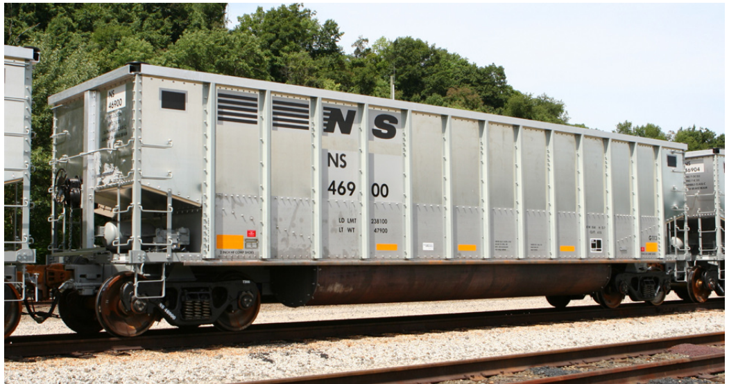
▲ One of the new batch of Freight Car America wagons, No. NS46900, pictured at Shire Oaks Yard. This is one of the fleet which is fitted with ECP control.. Eric M. Johnson
